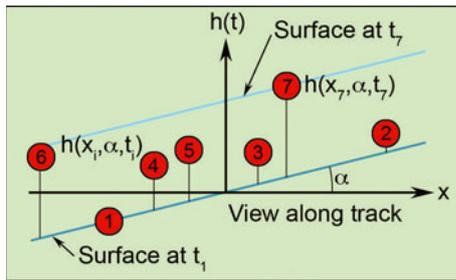
**Fig. 1.** Schematic of elevations  $h(x_i, \alpha, t_i)$  for successive data collected on repeat tracks at times  $t_i$  along an ICESat reference track with cross-track slope  $\alpha$  and distance  $x_i$  from the reference track.  $h$  is shown increasing with time.
