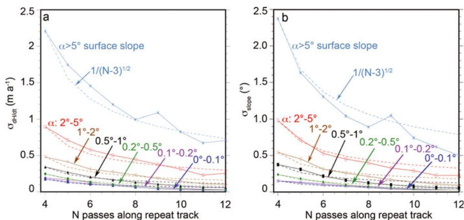
**Fig. 2.** (a) Error on ICESat  $dh/dt$  ( $\text{m a}^{-1}$ ) as a function of the number of repeats,  $N$ , used in the solution at each along-track location separated by 172 m.  $0.25 \text{ m a}^{-1}$  accuracy is achieved for  $N \geq 10$  repeats for slopes  $< 2^\circ$ . Dashed curves are  $1/(N-3)^{1/2}$  fits to the errors. (b) Error on slope  $\alpha$  as a function of  $N$ . Slope error is about  $\pm 20\%$  for  $N=10$ .
